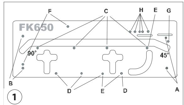
The steel stops are furnished with rubber rings which prevent the stops from dropping out of the holes. Place the metal stop into the hole using the pin with the rubber ring, so that it is completely inserted. If the metal stops are difficult to insert, lubricate the rubber rings with oil. Before using always ensure that the stops are completely inserted into the holes. Before using check that the stops are not leaning against the work table.
