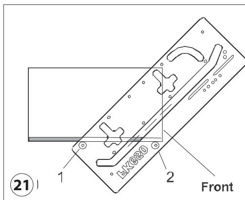
Insert the metal stops into the holes. Fix the jig FK to the edge of the worktop using the stops. Tighten the jig to the kitchen worktop using the clamps and check that the clamps do not hinder the movement of the router. Set the cutting depth on the router. Insert the router and begin to cut the joint on multiple-pass from left to right. Copy according to the outer edge of the radius or groove.
