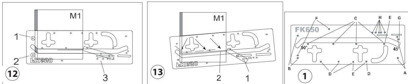
Tighten the jig to the kitchen worktop using the clamps and check that the clamps do not hinder the movement of the router and that the jig is well tightened to the kitchen worktop. Loosen and remove the sliding length stop to prevent its damage. Set the cutting depth on the router. Insert the router and begin to cut the joint on multiple-pass from left to right. Copy the far edge of jig FK (fig. 12).
