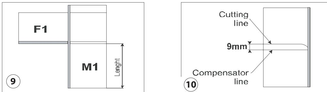
Remove the sliding length stop from the hole. Insert two metal stops into the B holes from the facing side of FK and place the FK onto worktop M1 (which is rotated upwards by its underside) by the facing side according to (fig. 11). Set the distant edge of the jig FK (see arrows) exactly according to the plotted compensatory cutting line.
